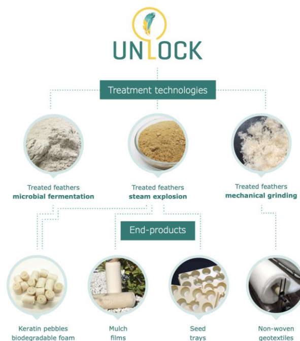
Figure 1. UNLOCK treatment technologies and end-products.
